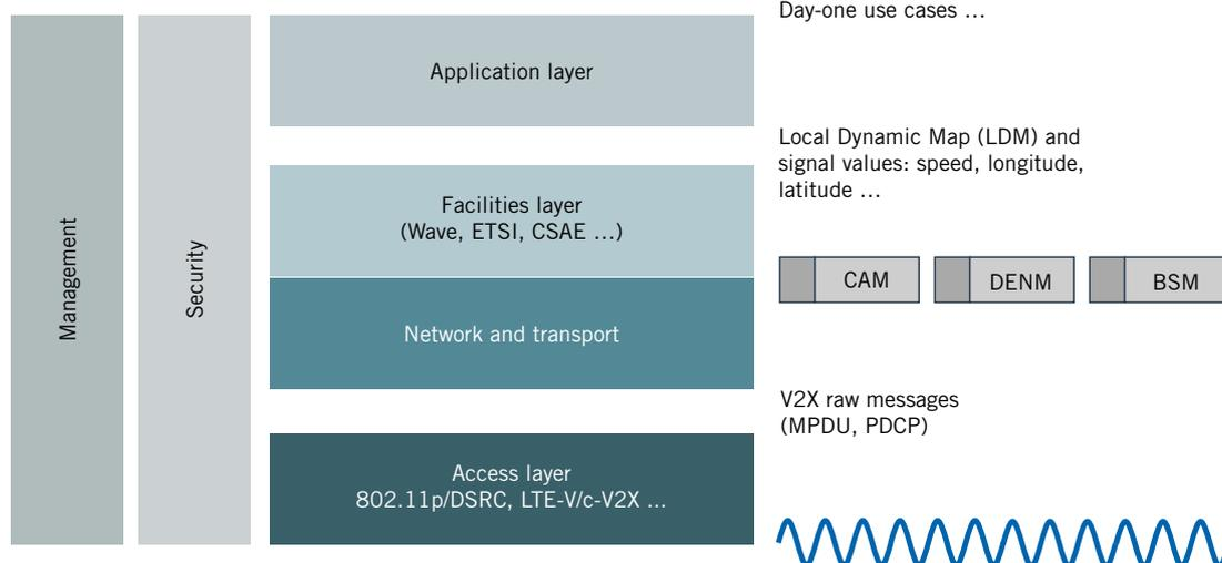
**FIGURE 1** Schematic layer structure of the V2X model (© S.E.A. Datentechnik)
