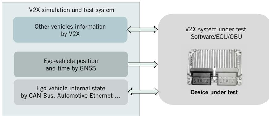
FIGURE 4 Test system for functional tests (schematic) © S.E.A. Datentechnik
