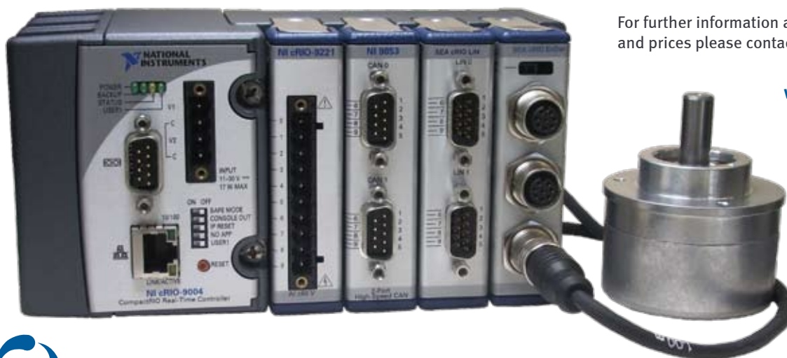
CompactRIO system with National Instruments IO and CAN module, S.E.A. LIN and EnDat module with HEIDENHAIN Drehgeber
