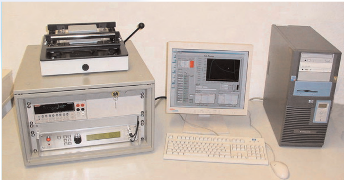
PC based IVL TEST PLATFORM with test adapter, 19" rack, including pulse generator, meter, multiplexer, stimulation, and measurement electronics
